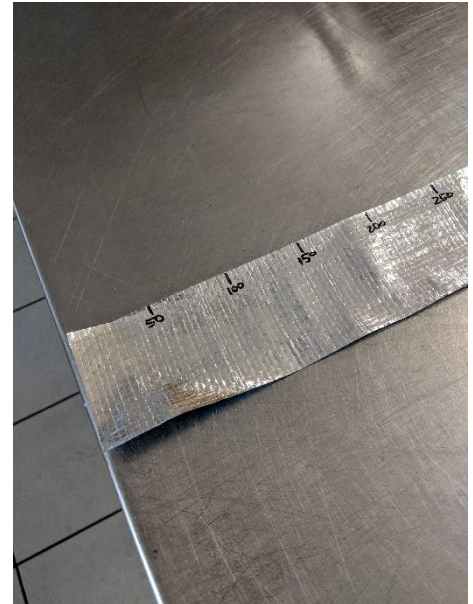
FIG.2 STRAPPING TAPE PREPARED FOR TESTING
